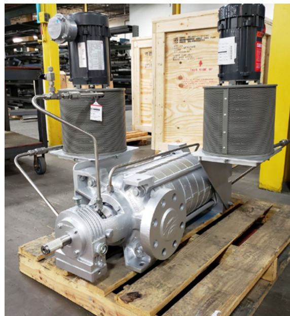
Air-cooled seal support system for applications where external cooling fluid is unavailable Plan 23
